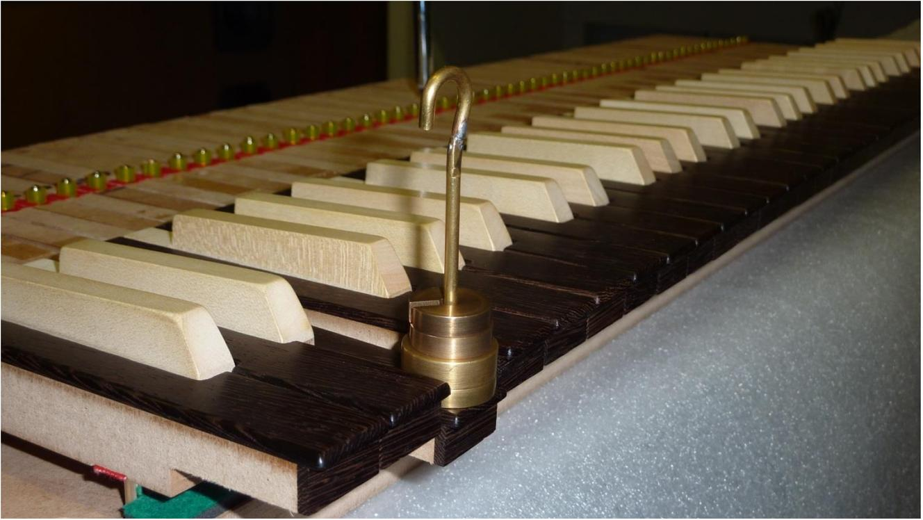
Testing and verify that the key stays on pressed position with 60g of weight.
