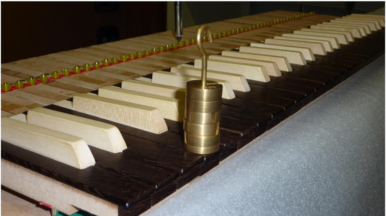
Testing and verify that the key stays on rest position with 120g of weight.
